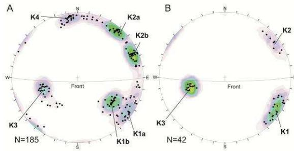
Fig. 3 – Stereographic projections of joints systems: poles from UAV-DTP (A); poles from DTP (manned helicopter) and geological engineering surveys (B)
