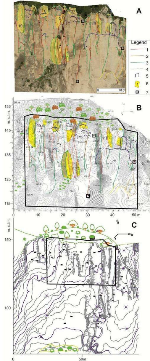
Fig. 2 –Photo by drone of Coroglio cliff and georeferenced (A) on the photogrammetric survey (B): 1) Open fracture (> 1cm wide); 2) Open fracture (0,05-1 cm wide); Closed fracture (< 0,05 cm); 4) Stratigraphic contact between fall pyroclastic deposits and tuff; 5) Rock fall source area; 6) Isolated unstable dihedral and rock pinnacle and referring number ; 7) Target; C) Photogrammetric survey by helicopter (year 2000). The box shows the studied area.
