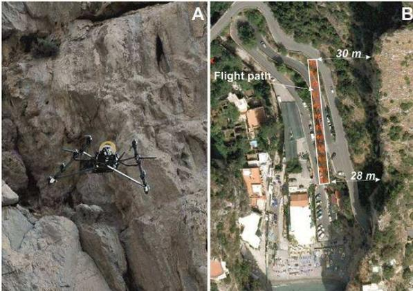
Fig. 1 – The drone and calibrated camera along the “Praiano” gorge (A); distance of the drone flight path from the rock cliff (B).
